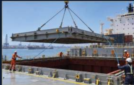
Hatch-cover lifting and placement
